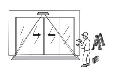
Normal mode When the sensor is powered, the green light flashes and output the door opening signal. When the sensor detects the stable background for 8 consecutive seconds, self-learning is successful. Green light is on and not output the door opening signal, sensor will enter the standby state.
