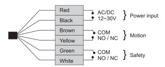
Note: 1, When connecting the wire, please don't tear the protection cover, as this may cause a electric leakage hazard or sensor failure
