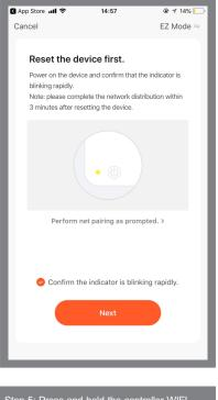
Step 5: Press and hold the controller WIFI learning button for 10s, WIFI blue light indicator is flashes, then check "Confirm the indicator is blinking rapidly" in the "tuya Smart" interface.
