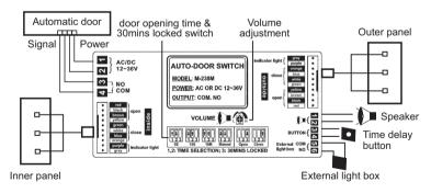
The inner and outer panel wiring are the same. Red, black, brown, yellow => Door open sensing port; Green, white, blue, orange => Door close sensing port; Purple, grey => LED indicator
