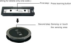
Attention: Since the system has learned the current sensing touch environment when the battery is installed, when fixing it to the wall, it may appear to be in the sensing status. Don't sensing or touch the panel at this time, after 16 seconds the system will re-learn the touch environment.
