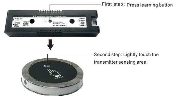
**Remark:** Since the system has learned the current touch environment when the battery is installed, when fixing it to the wall, it may appear to be in the sensing status. Don't touch the panel at this time, after 16 seconds the system will re-learn the touch environment.
