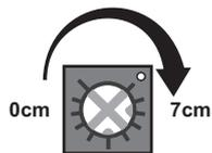
The clockwise direction the induction distance becomes farther, the counterclockwise direction the induction distance becomes closer, and the maximum induction distance is 7cm.
