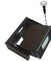
Fixed the mounting bracket first, and rotate the sensor body.
