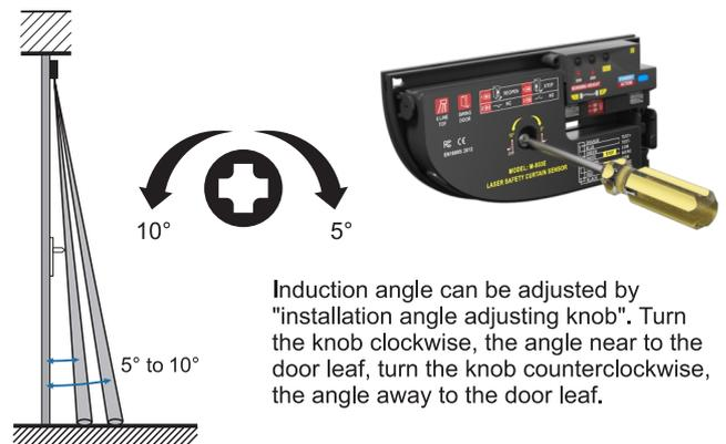
Induction angle can be adjusted by "installation angle adjusting knob". Turn the knob clockwise, the angle near to the door leaf, turn the knob counter-clockwise, the angle away to the door leaf.
