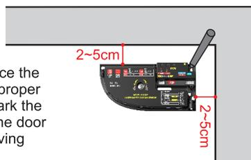
2. Drill the installing holes and threading holes for the master and slave machine in the door leaf.
