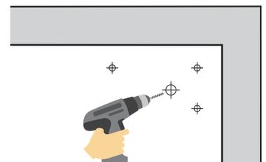
3. Tighten the screws to fix the sensor, connect the master and slave machine, then only one of them needs to be connected with the door opener. Or don't drill holes on the door, directly connect the master and slave machine to the door opener respectively.
